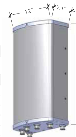
MANUF.: AMPHENOL MODEL: HTXCWW63111414 BAND: TRI BAND FREQ. (LOW): 696-960 FREQ. (HIGH): 1710-2170 POLARIZATION: ±45° WEIGHT: 13 LBS
